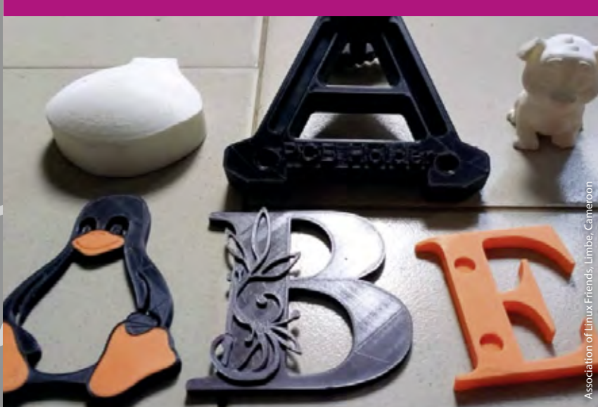
A selection of 3D printed items, produced from the plastic waste from discarded fishing gear and other plastic waste.
